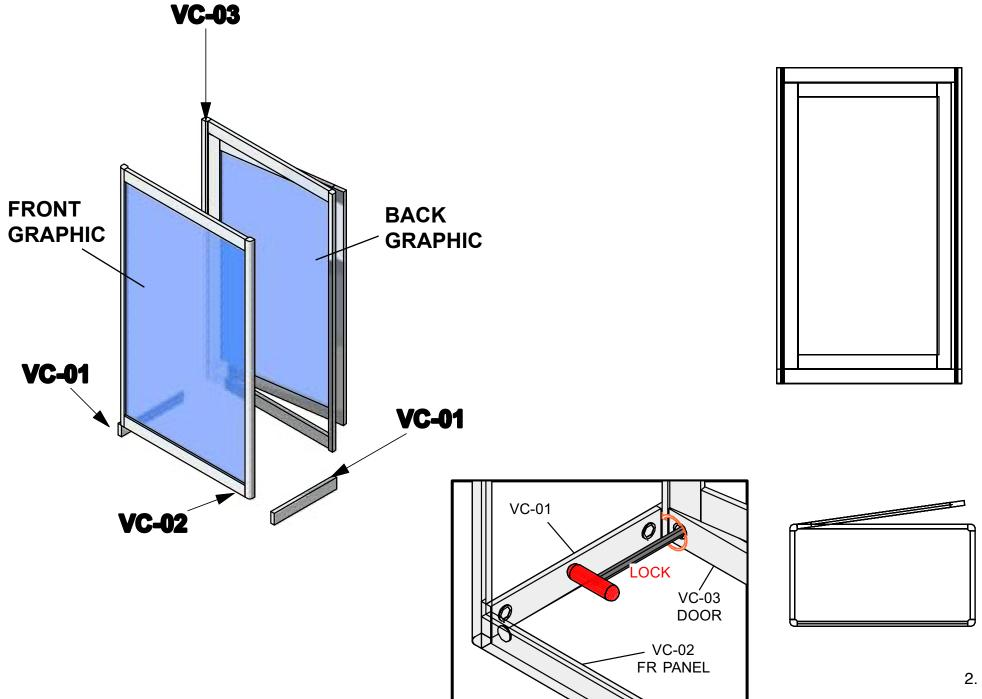
Step 2. Slide the side graphics into the VC-01s and secure in place by securing a VC-01 over the top in the graphic. Insert shelf supports using detail below and gently place internal shelf on the supports.
