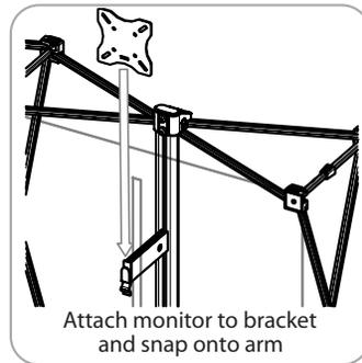
Attach monitor to bracket and snap onto arm
