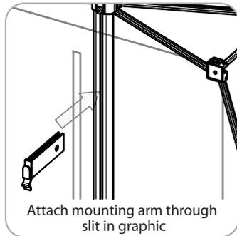
Attach mounting arm through slit in graphic
