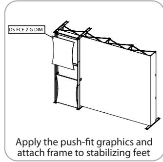
Apply the push-fit graphics and attach frame to stabilizing feet
