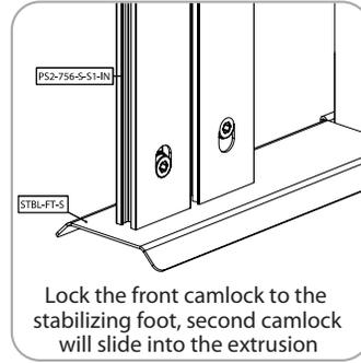
Lock the front camlock to the stabilizing foot, second camlock will slide into the extrusion
