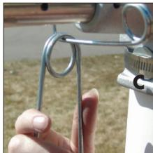
\*Pin should clip below casting
