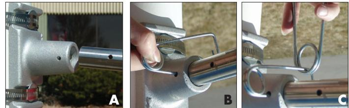
\*Pin should clip above casting
