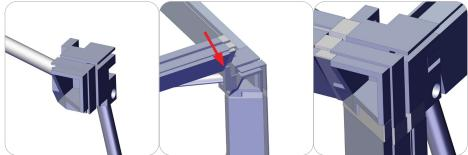
The scissor frames will have this corner hub installed on all four corners, front and back of the frame. This corner hub takes the end caps of the channel bars. The end caps of the channel bar will snap into place.
