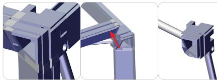
To remove the channel bars, start by pulling the end caps off the corner hubs.
