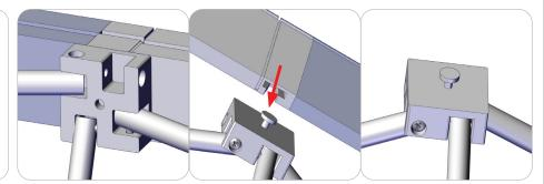
Continue to remove the channel bars by pulling the channel caps off the middle hubs.
