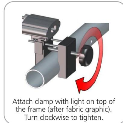
Attach clamp with light on top of the frame (after fabric graphic). Turn clockwise to tighten.
