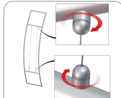
Twist on cables to top and bottom tubes.
