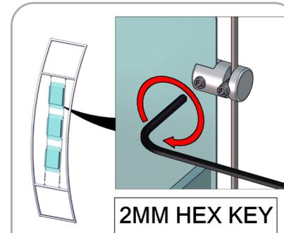
Install brochure holders on cables with CKP54 using 2mm hex key.
