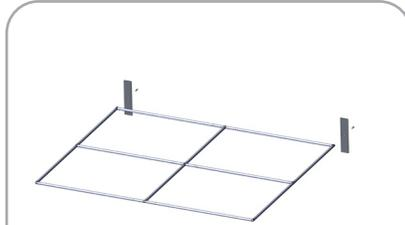
Once frame is connected attach feet. It is best to assemble with frame still laying flat.
