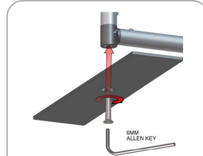
Use provided allen key, secure feet to bottom of frame by screwing bolt.
