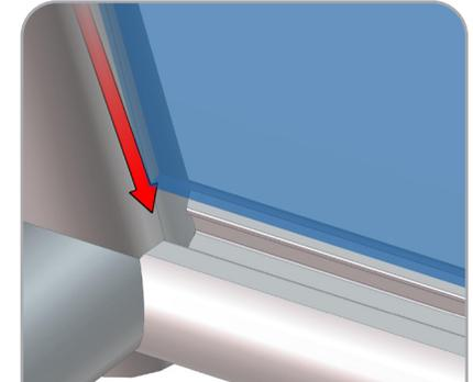
Slide infill panels into channels.
