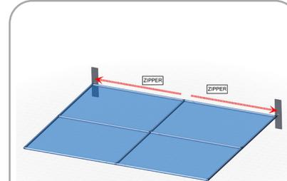
Slide graphic over top end of frame. Zip fabric closed on bottom.
