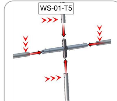
Use WS-01-T5 to connect frame in the middle; snap on button.
