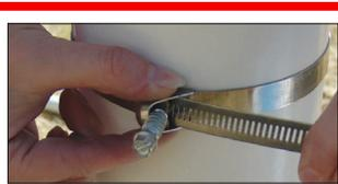
**DO NOT use a power tool to tighten the stainless steel bands! Over tightening will cause damage.**
