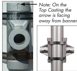
Secure the top Castings (1) to the Pole with two Stainless Steel bands (3). If attaching to a square or other shaped pole, it is recommended to use an additional set of bands, available separately. Tighten the bands until they hold the bracket securely and lock it into place with a screw or nut driver. Be sure the Band head is on the side of the pole and not on the casting. Clip off any excess band length.
