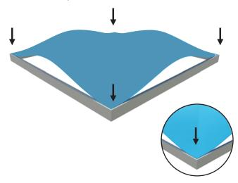
Push the siliconebead into the middle of the run and work your way around the perimeter of the frame until all beading is pushed in properly
